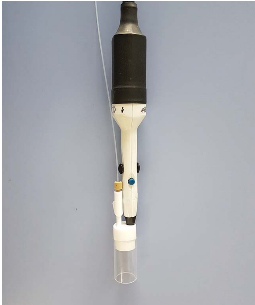
FIG. 1: J-Plasma handpiece with nebulizer and spray chamber
