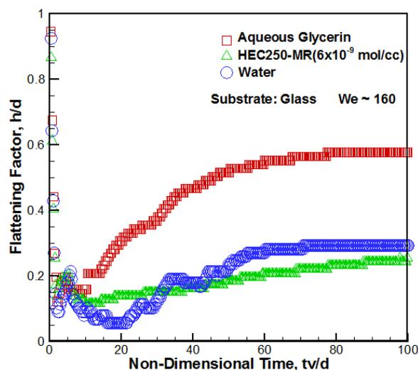
**FIG. 12:** Variation of flattening factor with nondimensional time. Glass substrate,  $We \sim 160$ .
