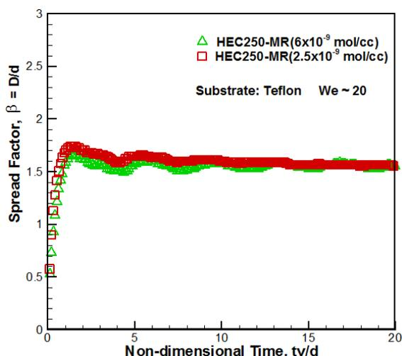
**FIG. 15:** Effect of polymer concentration on the variation of spread factor with nondimensional time. Teflon substrate,  $We \sim 20$ .
