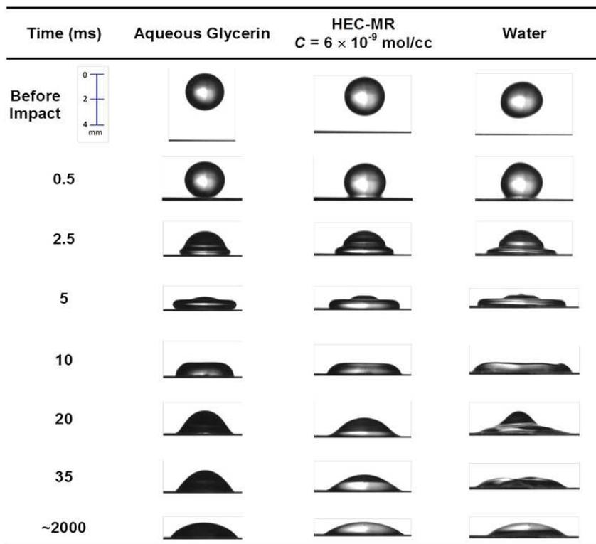
FIG. 5: High-speed photographs of drop spread on a glass substrate,  $We \sim 20$ .
