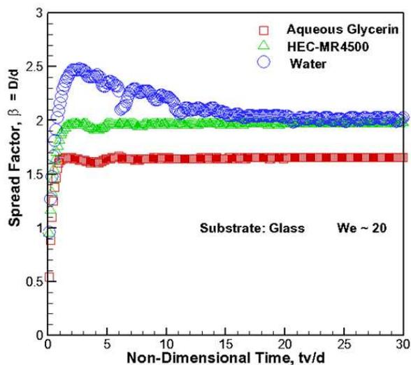
FIG. 6: Variation of the spread factor with dimensionless time. Glass substrate,  $We \sim 20$ .
