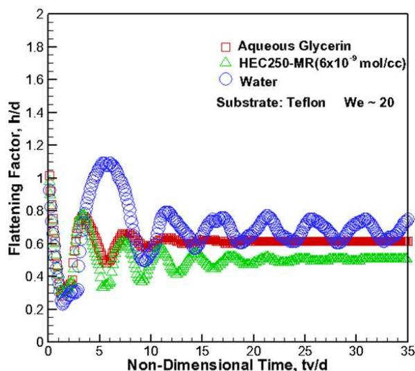
FIG. 10: Variation of the flattening factor with nondimensional time. Teflon substrate,  $We \sim 20$ .
