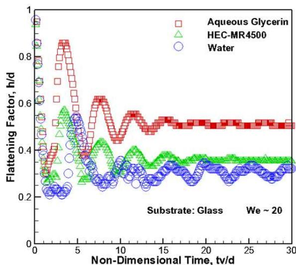
FIG. 7: Variation of flattening factor with nondimensional time. Glass substrate,  $We \sim 20$ .
