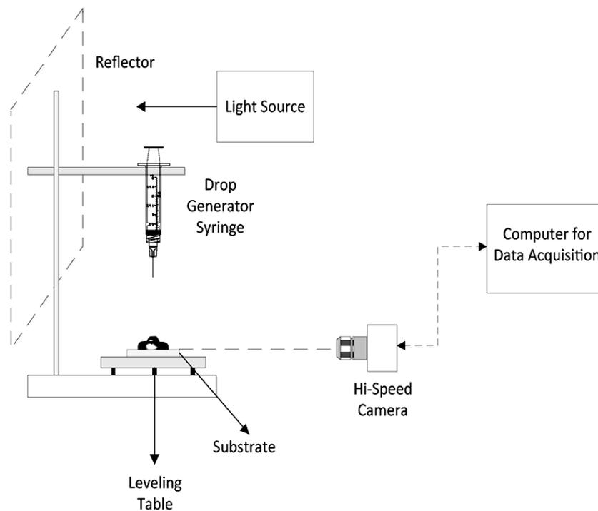
**FIG. 2:** Schematic of experimental data acquisition and analysis setup.
