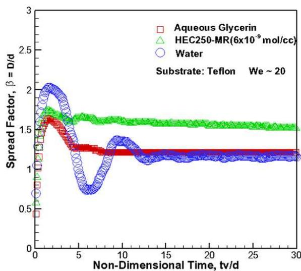
FIG. 9: Variation of the spread factor with nondimensional time. Teflon substrate,  $We \sim 20$ .
