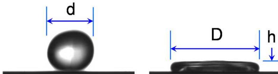
**FIG. 1:** Geometrical attributes of a droplet to characterize its spread and film height on a solid substrate.
