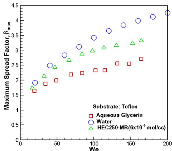
**FIG. 13:** Variation of the maximum spread factor (maximum uncertainty in  $\beta$ ,  $\pm 1.28\%$ ) on a Teflon substrate with Weber number.
