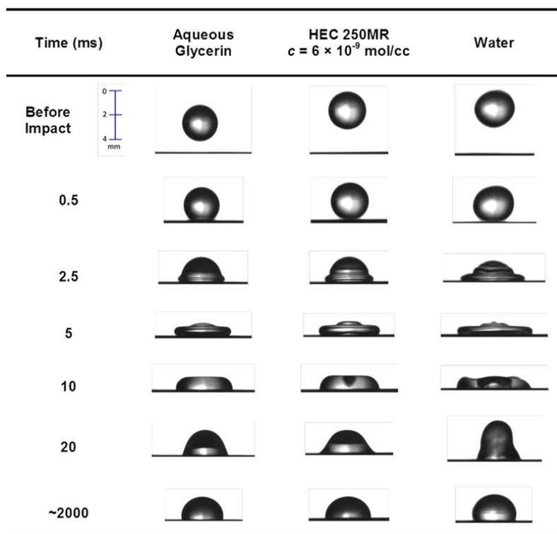
FIG. 8: High-speed photographs of drop spread on a Teflon substrate,  $We \sim 20$ .
