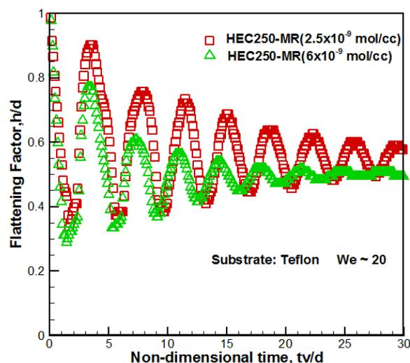
**FIG. 16:** Effect of polymer concentration on the variation of flattening factor with nondimensional time. Teflon substrate,  $We \sim 20$ .
