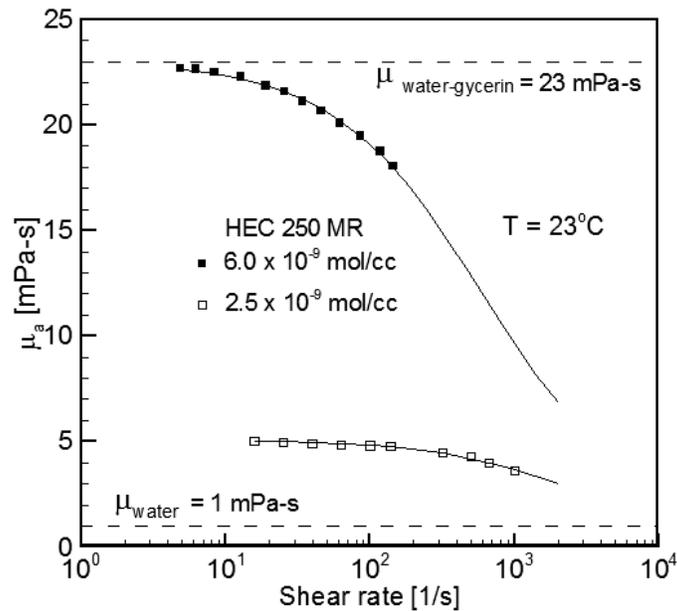
FIG. 4: Shear-dependent viscosity behavior for aqueous solutions of HEC 250 MR.
