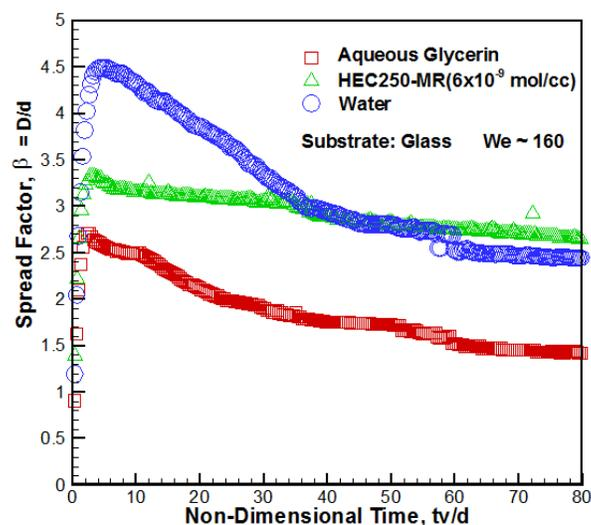
FIG. 11: Variation of spread factor with nondimensional time. Glass substrate,  $We \sim 160$ .
