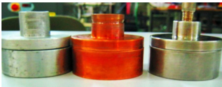
FIG. 2: Different types of metal electrodes: stainless steel, copper and aluminum
