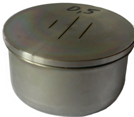
FIG. 1: A process challenging device: a metal box with 3 slits of 0.3 mm width.
