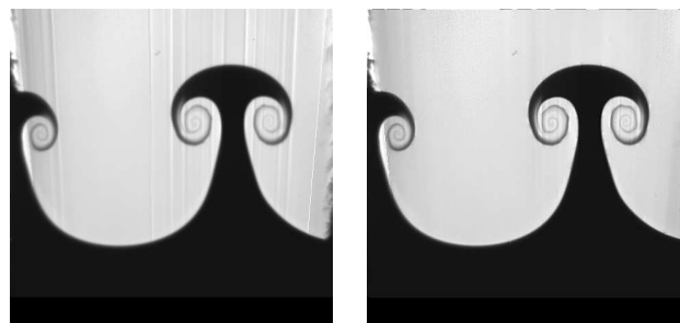
FIG. 2: Reducing domain-specific noise in images from experiments of Richtmyer-Meshkov instability. Left: original image; right: after reducing the noise that appears as vertical lines in the image.
