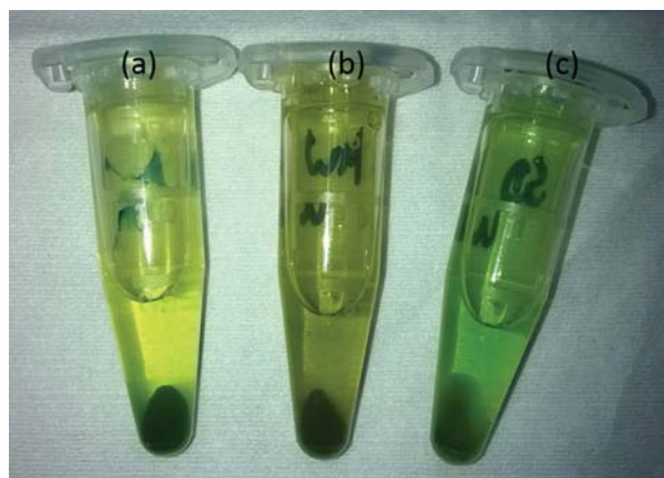
FIG. 14: Color images of extracted pigments for untreated control (a), after microwave exposure (b), and after spark discharge treatment (c). The dark objects at the bottom of the tubes are the centrifuged algae pellets.
