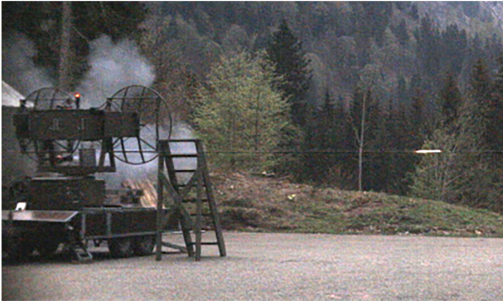
FIG. 16: The exhaust trail on the right of this video frame demonstrates fast ignition (Reprinted from Veraar and Mayer, 2006)
