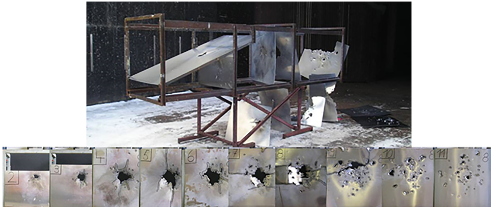
FIG. 17: Impact damage on a range target representing a fighter aircraft (Reprinted from Veraar et al., 2006)
